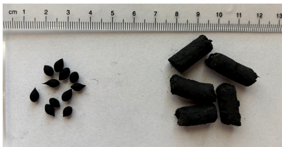
Fig. 1. Activated carbon seed coatings (left) and pellets (right) used to protect seeded species from herbicide toxicity.
