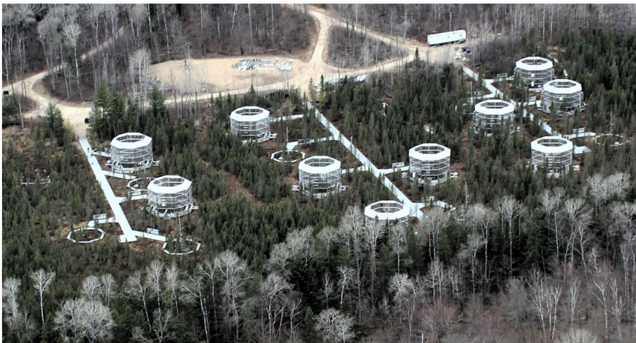
Photo: Oblique aerial view of the Marcel SPRUCE project in northern Minnesota, April 2015. Each enclosure is 12 meters in diameter, 8 meters tall, and extends about 2 meters below the peatland surface. Photo courtesy of Oak Ridge National Labs.
